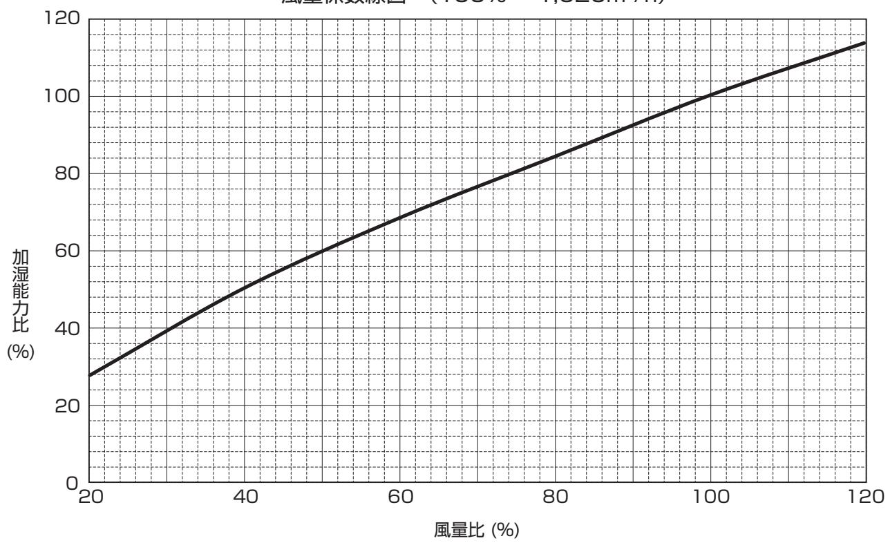
**PFAV-P140DMJ1 組込 WM-VPH0305MD**加湿能力線図（空調機風量 2,700m<sup>3</sup>/h 時）
